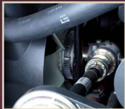
Electro magnetic radiator fan auto clutch (Powertec engine)
